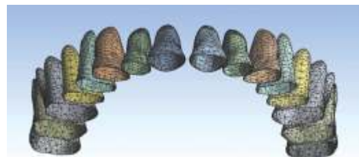
Fig 2. FEM Model of Periodontal Ligament
